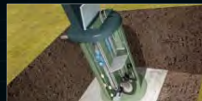
Installation options include submerged installation on auto-coupling with guide rails.
