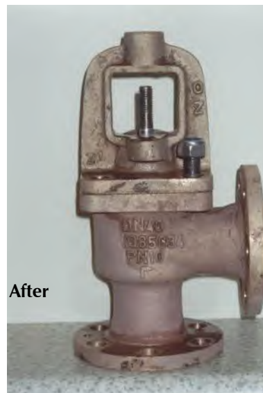
After agitation in TRIPLE 7 Heavy Duty and TRIPLE 7 Enviroscale baths.
