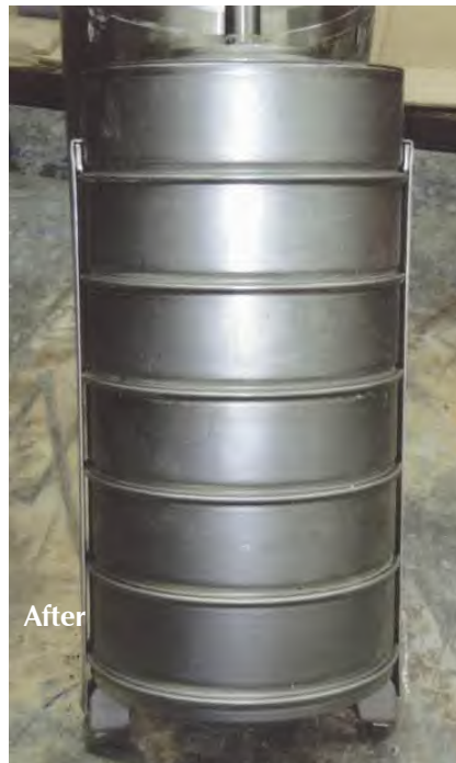
Soaked in a 10% solution of TRIPLE 7 Enviroscale overnight.
