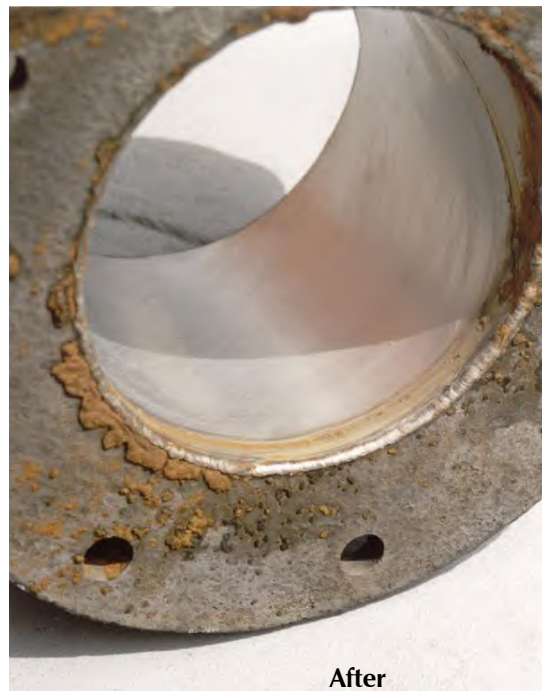
TRIPLE 7 Enviroscale in an agitated bath was applied for approximately 7 hours.
